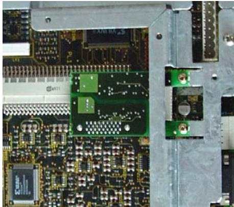
Figure 3-8 DELTA System - final position of the CAN 2 Board
