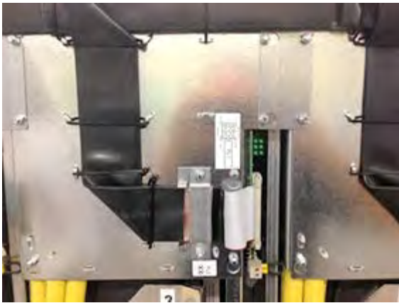
Figure 5-11. – Ribbon Cable Clamp At The DELTA Transistor Module
