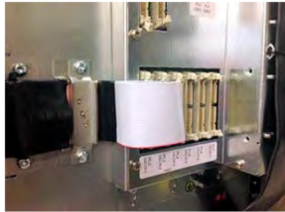
Figure 5-12. – Ribbon Cable Clamp At The DELTA Controller
