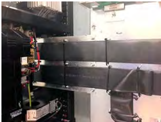
Figure 5-13. – Typical Ribbon Cable Routing Across The DELTA Transistor Modules
