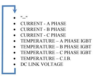
• In a similar manner to the analog outputs, most values are displayed as the percentage of a defined value. The exception is the C.I.B. temperature which is displayed in °C.
