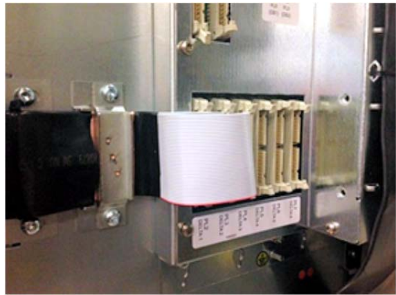
Figure 5-17. – Ribbon Cable Clamp At The DELTA Controller
