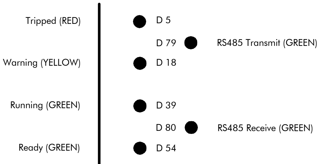
Figure 8-2 Functions of LEDs for MV3000e Controller for DELTA Modules
