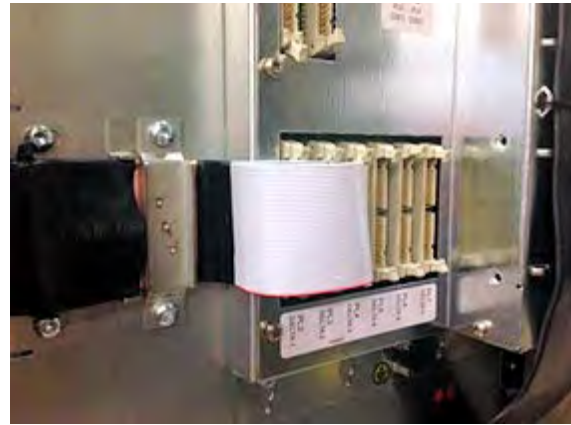
Figure 5–17. – Ribbon Cable Clamp At The DELTA Controller
