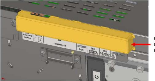
PRESS HERE TO DISENGAGE PROTECTOR FROM COVER
