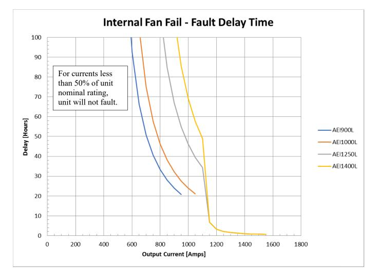
• The following figure shows the fault delay time as a function of the load current:
