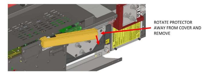
• This protector should be kept safe and re-fitted if it is ever necessary to remove the AEI unit.
