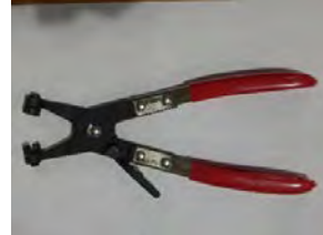
Pic.5 Special key for hose clamp
