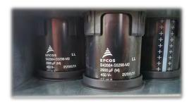
After long periods of storage, these capacitors will eventually 'de-polarize' and become ineffective. The effects of this are difficult to predict as too many variables are involved. However, the symptoms could include random or spurious trips, power supply failures or extreme levels of ripple on the DC bus. Excessive capacitor leakage could also lead to overheating of pre-charge resistors.
