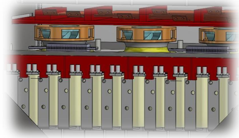
The fans in the 3.6 MW nacelle converter operate in the harshest environment due to the proximity of high DC currents both above and in front of the fan plate assembly. There is often a presence of brake dust near the fans.
